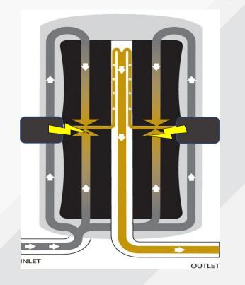
Magnetics improves 1-Micron depth-media filter capacity by 15-30%
